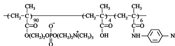
Figure 1 Chemical structure of photo-reactive phospholipid polymer, Az-PMAc.
