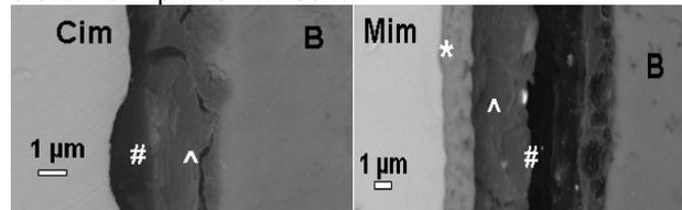
FE-SEM analysis of interfacial bonding fracture at the bone to implant interface. Cim = control implant, Mim = Mg implant, B = bone, \* = oxide layer, # = fractured space during mechanical loads/RTQ testing, ^ = amorphous immature bone layer.
