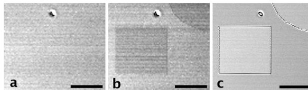
**Figure 1.** a) Fresh photoresist, b) DIC imaging after exposure, and c) developed master. Scale Bar = 50  $\mu\text{m}$ .
