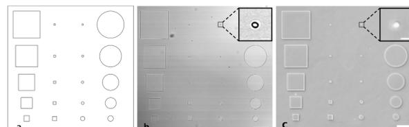
**Figure 2.** a) Virtual mask, b) developed master, and c) replica-molded PDMS stamp. Scale bar=100  $\mu\text{m}$ . The minimum feature size achieved with a 10 $\times$  objective (NA 0.45) was 3  $\mu\text{m}$  (enlarged in b,c; scale bar=5  $\mu\text{m}$ ).
