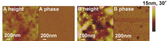
Figure 1. Tapping mode AFM height and phase images of PTMC films before treatment (A), and after immersion in lipase solution at  $37^\circ\text{C}$  for 1 min (B).
