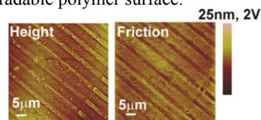
Figure 2. Contact mode AFM height and friction images of PTMC films after  $\mu$ CP using lipase solutions.
