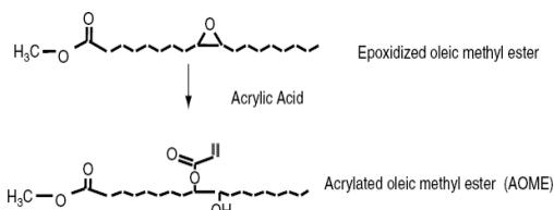
**Figure:** Structure of the plant oil derived monomer AOME.
