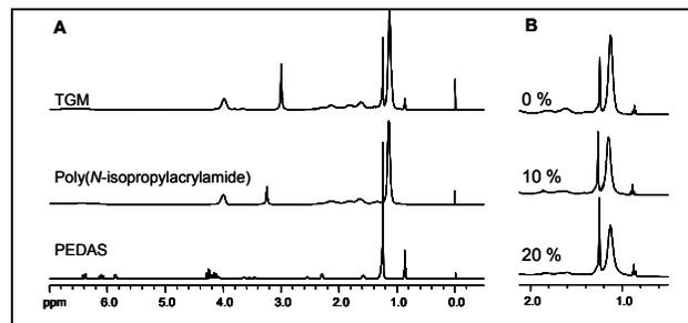
Figure 2:  $^1\text{H-NMR}$  spectra: A: TGM and structural components.
