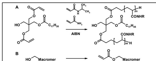
Figure 1: A: Synthesis of TGM (R: -H or  $-\text{CH}(\text{CH}_3)_2$ ).
