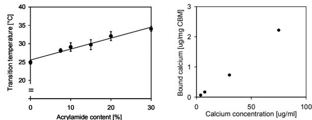
Figure 3: Onset temperatures of the phase transition of TGMs with different AAM contents ( $n=3$ ).
