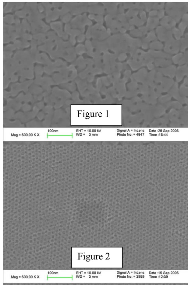
**Conclusions:** The mechanical and optical characteristics of nanoporous titanium dioxide films can be adjusted to fit specific requirements in terms of porosity, index of refraction, thickness and crystalline morphology by employing the synthesizing conditions described herein. Therefore, by tailoring film characteristics we anticipate being able to match drug delivery requirements to specific films characteristics.
