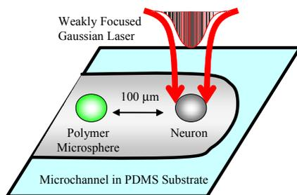
To fabricate a spin-coated Poly Dimethyl Siloxane (PDMS) surface a mold was created by photolithography. Shallow channels (~30  $\mu$ m depth) were created to confine the neurite outgrowth regulated by the NGF diffusion in 1D as shown (Fig. 2).
