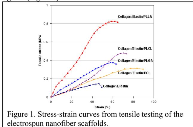
Figure 1. Stress-strain curves from tensile testing of the electrospun nanofiber scaffolds.
