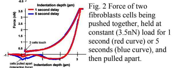
Fig. 2 Force of two fibroblasts cells being pushed together, held at constant (3.5nN) load for 1 second (red curve) or 5 seconds (blue curve), and then pulled apart.
