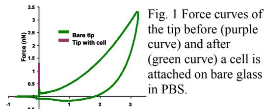
Fig. 1 Force curves of the tip before (purple curve) and after (green curve) a cell is attached on bare glass in PBS.
