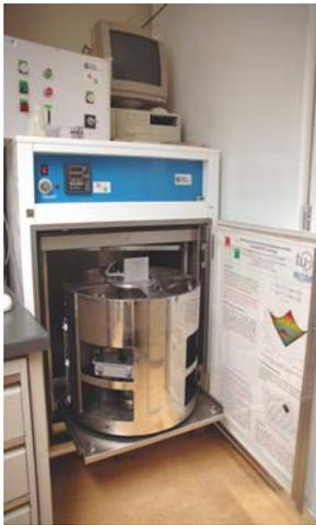
Fig. 1 Medium Size Centrifuge for Acceleration Research used to simulate hypergravity.
