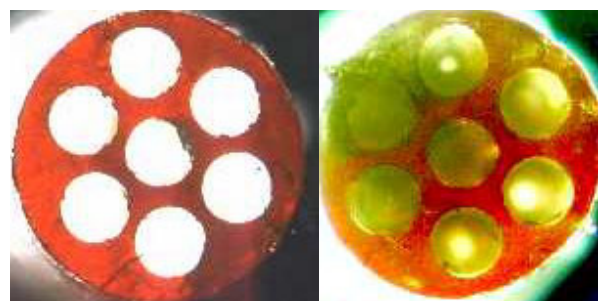
Fig 2: Representative pictures of day 0 (left) and week 12 (right) PCLF multi-channel scaffolds.
