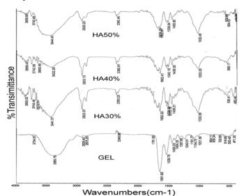
Fig. 1. FT-IR spectra for GEL and 30wt%, 40wt%, 50wt% cross-linked HA-GEL composites
