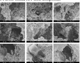
Fig.2. SEM micrographs of the pores in the cross-section of different HA-GEL scaffolds (a)HA30% (b) HA40% (c)HA50%
