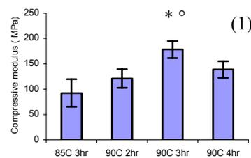
Fig 1 Mechanical properties of PLAGA/HA 4 to 1 scaffold at different sintering temperature and time. (\*) and (o) indicate significant difference comparing different sintering temperature and time.
