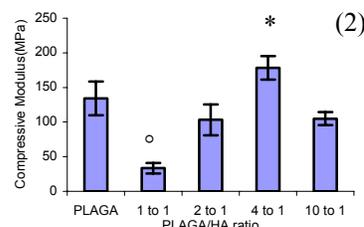
Fig 2 Mechanical properties of different compositions of scaffolds. (\*) indicates significantly higher than all the others. (o) indicates significantly lower than all the others.
