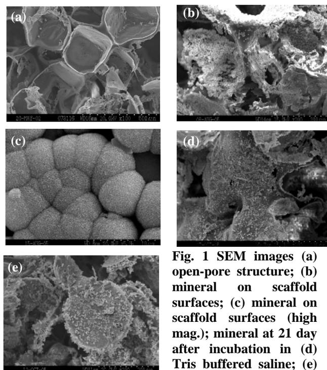
**Fig. 1 SEM images (a) open-pore structure; (b) mineral on scaffold surfaces; (c) mineral on scaffold surfaces (high mag.); mineral at 21 day after incubation in (d) Tris buffered saline; (e) cell culture media**
