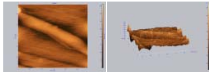
Fig. 3 AFM image of pure collagen type II fiber and collagen II-HA copolymer
