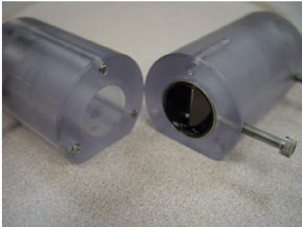
In addition we have developed a customized chamber to test fully assembled heart valves and to compare with those manufactured by different companies.
