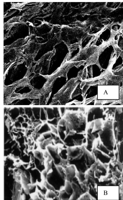
Fig 1A and B show SEM pictures of degraded chitosan scaffold before degradation and 4 weeks after degradation with lysozyme respectively at x30k and 20kV acc. voltage
