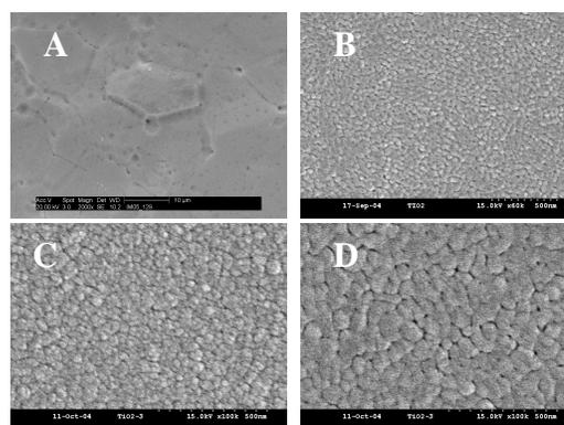
Fig.1 Representative surface morphology. A) Ti; B) As-deposited TiO<sub>2</sub>; C) 400°C heat-treated TiO<sub>2</sub>; and D) 600°C heat-treated TiO<sub>2</sub>. bar = 500nm
