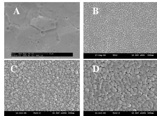
Fig.1 Representative surface morphology. A) Ti; B) As-deposited  $TiO_2$ ; C) 400°C heat-treated  $TiO_2$ ; and D) 600°C heat-treated  $TiO_2$ . bar = 500nm
