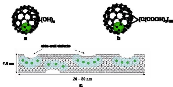
**Figure 1.** Depiction of (a) Gd@C<sub>60</sub>(OH)<sub>x</sub>, (b) Gd@C<sub>60</sub>[C(COOH)<sub>2</sub>]<sub>10</sub> and (c) a single Ultra short tube (US-tube) loaded with hydrated Gd<sup>3+</sup> ions (Gd<sup>3+n</sup>@US-tubes). In the case of US-tubes Gd<sup>3+</sup>-ion loading is likely through side-wall defects created by cutting full-length nanotubes to produce US-tubes (not to scale and Cl-anions and atoms attached to dangling C bonds not shown).
