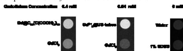
**Figure 2.** T<sub>1</sub> weighted MRI phantoms of the (a) Gd@C<sub>60</sub>[C(COOH)<sub>2</sub>]<sub>10</sub> and (b) Gd<sup>3+n</sup>@US-tubes solutions at 0.4 mM and 0.04 mM gadolinium concentrations, respectively, with a 1.5 T Philips MR imager. For comparative purposes MRI phantoms of pure water and 1% SDBS solutions are also shown.
