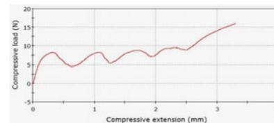
Fig. 3 Compression curve of a sintered scaffold
