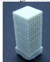
Fig.2 A photo of a sintered scaffold
