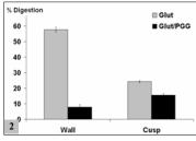
treatment significantly (p < 0.05) increased resistance to elastase of Glut-fixed aortic wall and cusp (Figure 2).
