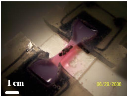
Figure 1. Type-I collagen, notched tensile specimen used to establish a mechanical strain gradient *in vitro*.
