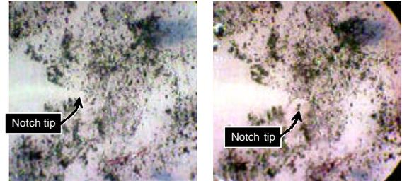
Figure 2. Optical micrographs of the notch tip region at low strain (left) and high strain (right).
