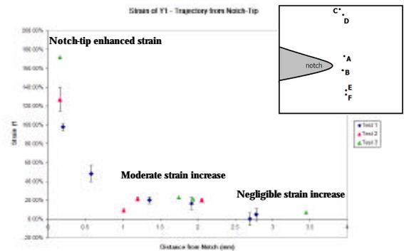
Figure 3. Mechanical strains vs. distance from the notch tip (Fig. 2).
