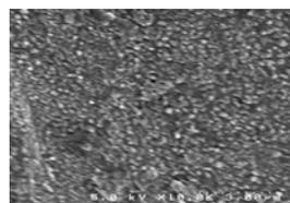
**Figure 2:** SEM image of a surface modified with gold nanoshells ( $10^4\times$ )
