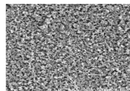
**Figure 3** SEM image of a surface modified with PS-NP 5000x
