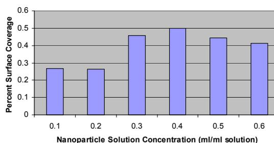
**Figure 1** PS-NP surface coverage. 20 minute dipping times and 0.4 % nanoparticle solutions produced the most surface coverage.
