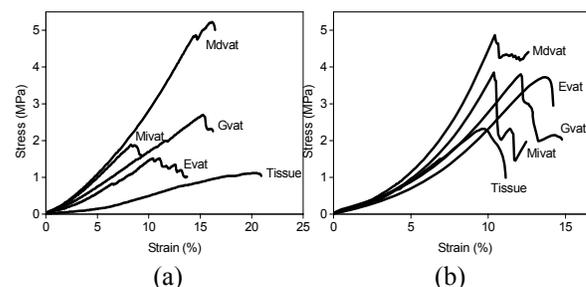
Figure 2. Stress-strain curve of respective bioscaffold. (a) longitudinal and (b) circumferential.
