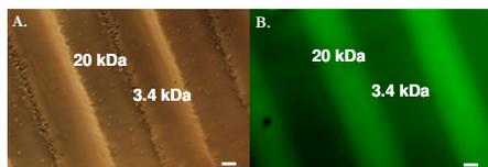
**Figure 1:** (A) Striped patterned PEGDA hydrogel. Surface patterning controlled by photomask geometry. (B) Patterning confirmed by exclusion of fluorescently-labeled 70 kDa dextran from stiffer stripes.
