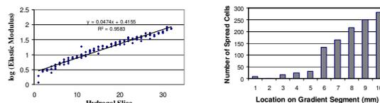
**Figure 3:** (left) Tensile testing of sequential sections of gradient hydrogel confirms a gradient of elastic moduli. (right) Analysis of cell location after 12 hr on gradient hydrogel shows SMC density increasing with stiffness.
