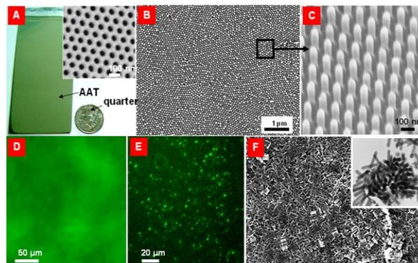
Figure 1. Manufacturing of rod shaped nanoparticles: A) nanoporous anodic alumina template; B) and C) SEM images of the molded SU-8 pillars; D) Fluorescence images of nanorods doped with green dyes before release from substrate and E) after release to aqueous solution; F) SEM image of massive rods produced (inset is TEM).
