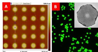
Figure 2. Manufacturing of disc shaped SU-8 particles: A) AFM of disc particles (2  $\mu\text{m}$  in diameter and 100-200 nm in thickness) on sacrificial polymer layer; B) fluorescence image of released disc particles encapsulated with SPIOs and green dyes. The inset is a TEM image of individual disc particles with uniform and dense distribution of SPIOs.
