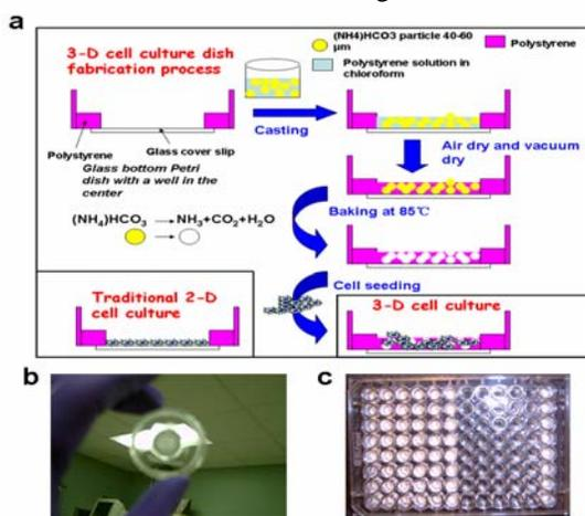
Fabrication and characterization of 3D cell culture vessels. (a): Schematic of the fabrication process. (b): Outlook of a 3D cell culture dish with a 3D polystyrene scaffold in the center. (c): Outlook of a 3D cell culture 96-well plates with 3D polystyrene scaffolds in the left half of the columns.
