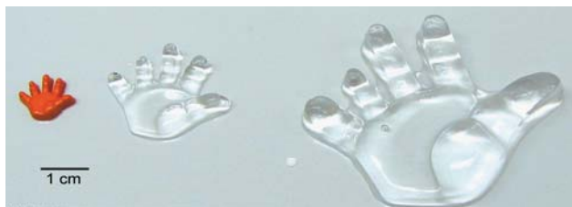
Figure 1. Images of chemically crosslinked super-swelling hydrogels of hyaluronic acid demonstrating the ability to maintain shape during swelling. Hand-shaped button that was used to cast the PDMS mold (left), hydrogel after swelling in saline (middle), and hydrogel after swelling in water (right). Scale bar = 1 cm.
