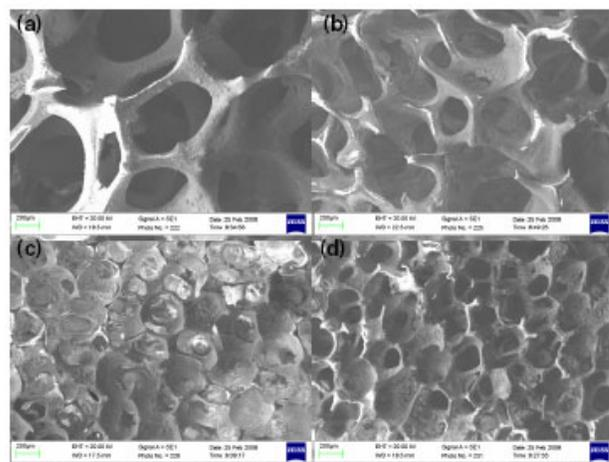
Figure 1. SEM images of the (a) 450 (b) 340 (c) 250 and (d) 200 μm pore size hydroxyapatite scaffolds
