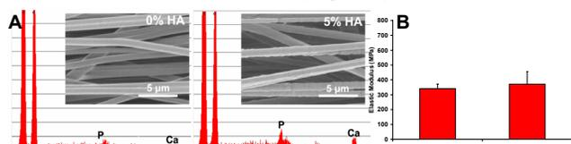
Fig. 1: A) SEM micrographs (4000x) and EDAX spectra of 0% and 5% HA nanofiber scaffolds, B) Yield strength of 0% and 5% HA scaffolds.
