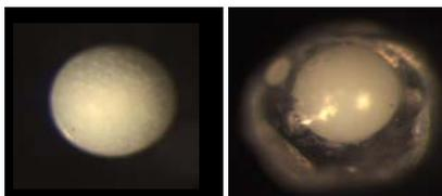
Figure 1. Uncoated (left) and coated (right) polymeric microsphere.
