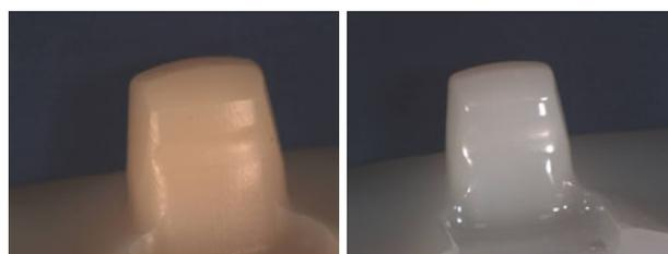
Figure 3. Representative Photos of the Impingement Regions of the Vitamin E Infused (Left) and Control (Right) Tibial Bearings After 3 Million Cycles of Cyclic Loading
