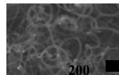
Figure 1. SEM micrograph of MWCNT-Ti.
