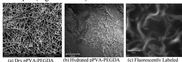
**Figure 1.** Electrospun pPVA-PEGDA fibers (a) dry (100 μm), (b) hydrated (100 μm), and (c) fluorescently labeled hydrated fiber network (20 μm).
