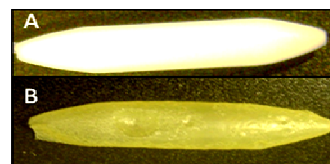
Figure 2. Derlin mold (A) used for fabrication of hollow polymer pouch (B).
