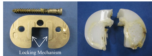
Figure 2. CoCr tibial tray with its corresponding polyethylene insert, fractured through the screw hole in the bridge
