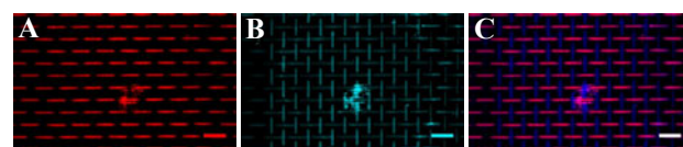
Figure 2: (A) OEG-terminated alkanethiols were desorbed from the surface, backfilled with biotin-terminated alkanethiols, and labeled with streptavidin-AF633. (B) A second cycle of desorption and biotin backfilling with streptavidin-AF568 led to some non-specific adsorption to the pattern in A. (C) Merge of A and B. SB = 10 \mu\text{m} .
