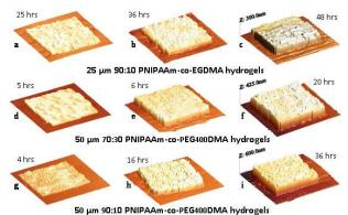
Figure 2. Normalized AFM images of patterned hydrogels showing spatial XY patterns and Z controlled hydrogel growth
