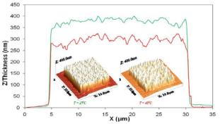
Figure 3. Thickness profile depicting responsive behavior of 25µm 90:10 PNIPAAm-co-PEG400DMA hydrogel at 40°C (green), and 25°C (red), and the respective normalized 3-D AFM images (inlays a & b)
