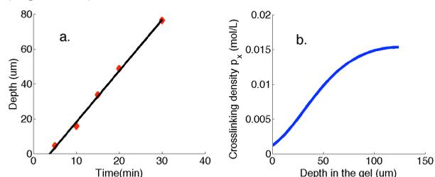
**Figure 2:** a. Depth of eroded channels as a function of exposure time. b. Crosslinking density as a function of depth within the gel.
