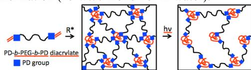
**Figure 1:** Photodegradable networks were formed by radical chain polymerization of PD-*b*-PEG-*b*-PD diacrylate and degraded by light exposure.
