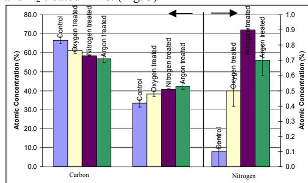
Figure 3. Atomic concentration of carbon, oxygen and nitrogen on PLA films (blue:control, beige:O<sub>2</sub> treated, purple:N<sub>2</sub> treated, green:Ar treated)
