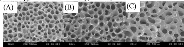
Fig 1. SEM micrographs of the porous Ti scaffolds(10 Vol.% of  $\text{TiH}_2$  contents) produced with various casting times of (A) 1 day (B) 3 day (C) 7 day
