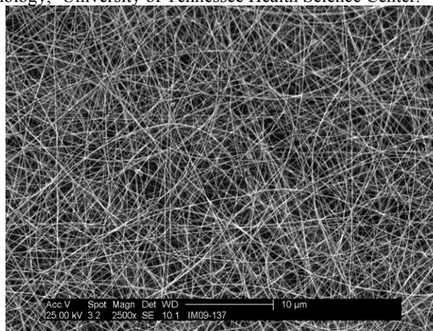
Figure 1 – SEM image at 2500X of nanofibers before neutralization.
