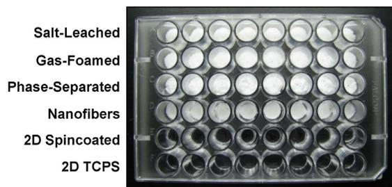
Fig. 1: Picture of 48-well platform for screening cell function on scaffolds with different topologies.
