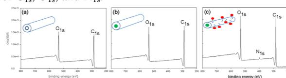
Figure 2. X-ray photoelectron scattering (XPS) spectroscopy of (a) NF, (b) bFGF NF and (c) bFGF/EGF NF.
