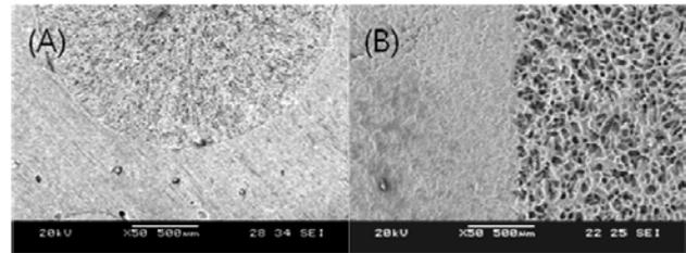
Fig 1. SEM micrographs of the porous HA scaffolds with dense shell; cross section of (A) radial direction (B) axial direction
