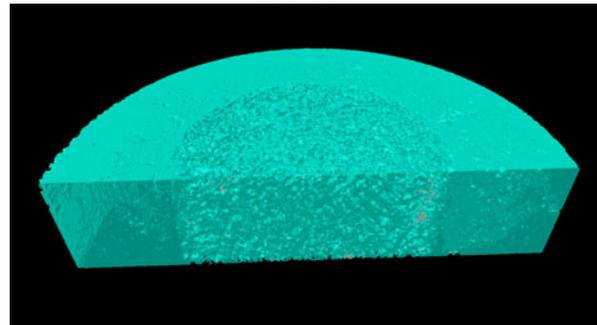
Fig 2. 3-D reconstruction of HA scaffolds using the micro-CT
