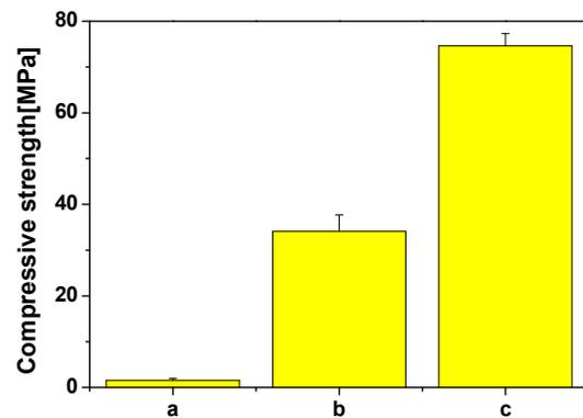
Fig 3. Compressive strength of the porous HA scaffolds ((a) scaffold fabricated using 10vol% slurry (b) scaffold fabricated to have same porosity with c using appropriate slurry (c) scaffold with dense shell fabricated using 10vol% slurry)
