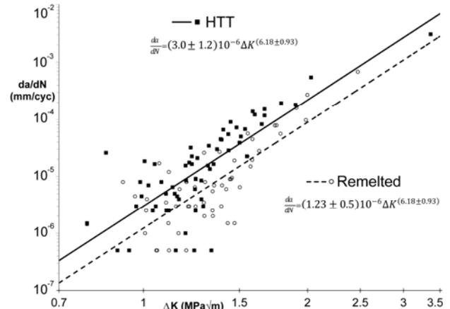
Figure 1: Fatigue crack propagation of high temperature treated and remelted ultra-high (with approximate bounds of 95% confidence interval)
