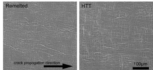
Figure 2: 300X magnification SEM images of the fractured surface of the remelted and HTT ultra-high.
