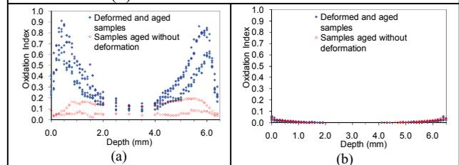
Cyclic loading, which has also been absent from standard accelerated aging techniques, also accelerated the oxidation of irradiated/melted UHMWPE (Fig 3a) and did not cause oxidation in irradiated, vitamin E-stabilized UHMWPE when tested for 5 million cycles (Fig 3b).
