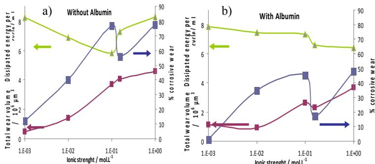
Figure 1. Dissipated energy per cycle / mJ; Total wear volume /  $10^6 \mu\text{m}^3$ ; % corrosive wear according to the ionic strength /  $\text{mol.L}^{-1}$ ; Ringer and NaCl solutions; a) without albumin, b) with albumin, 1 g.L<sup>-1</sup>.
