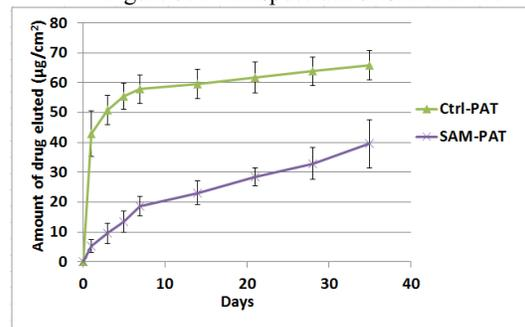
Figure 4. *In vitro* drug release profiles of SAM–PAT and Ctrl–PAT for  $100 \mu\text{g}/\text{cm}^2$  drug dose.
