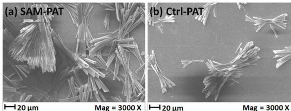
Figure 1. SEM images of PAT crystals on (a) SAM–PAT (b) Ctrl–PAT.
