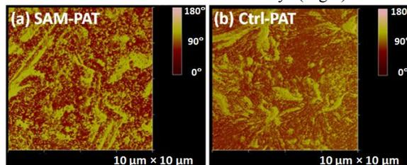
Figure 2. AFM tapping mode phase images of PAT molecular coatings on (a) SAM–PAT (b) Ctrl–PAT.
